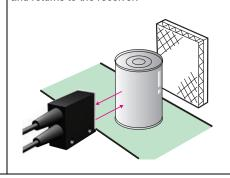
The light from the emitter hits the Reflector and returns to the receiver.
