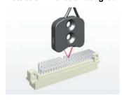
These Fiber Units detect only objects in the sensing range. Objects in the background that are located beyond a certain point are not detected.
