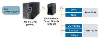
An AC-AC UPS is the optimum option for backing up devices with an AC input power supply.
