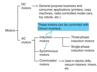
As induction motors can be used to achieve simple speed control at a relatively low cost, they are used in many applications. They can be operated just by connecting an AC power supply, so installation is extremely easy. Generally, a cooling fan is attached to the back to help dissipate heat generated by the motor.
