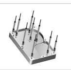
Measuring Warp in HDD Chassis Measurement time can be greatly reduced by using the multi-point measurement function.
