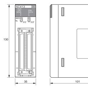
Note: The above diagram is for the CS1W-NC413.
